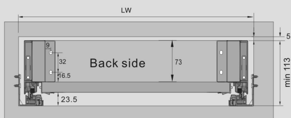
Drawer back installation dimensions
