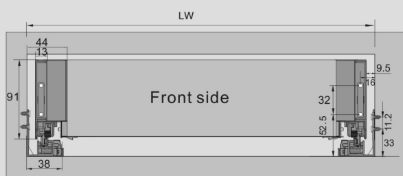
Drawer back installation dimensions
